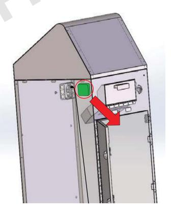
INSERT 4 AA BATTERIES, CLOSE CASE. REATTACH BATTERY CASE.
